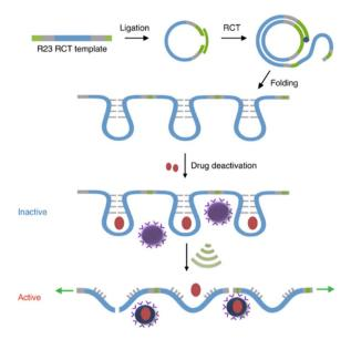
Fig. 6 Preparation of R23 polyaptamers by RCT from circular template and antibiotic releasing mechanism based on US-induced stretching and scission. Reprinted with permission from ref. 61. Copyright the authors under exclusive license to Springer Nature Limited.
