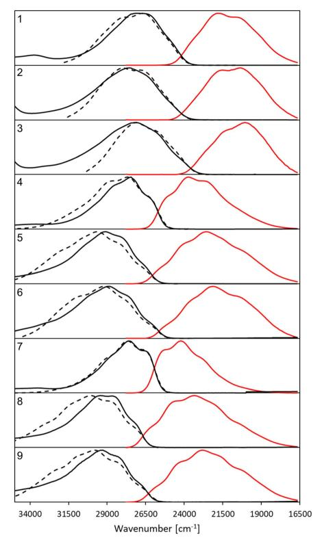
Fig. 2 Normalized, corrected absorption (solid black line), fluorescence (solid red line) and mirror-image of fluorescence spectra (dashed black line) shifted to match the 0-0 point in CHCl<sub>3</sub>.
