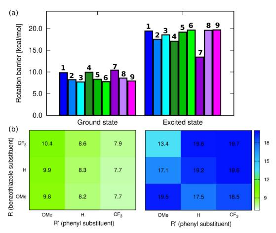
Fig. 4 (a) Barriers for rotation around the C15–C17 bond computed at the PCM(CHCl $_3$ )-(TD-)MN15/6-311++G(d,p)) level for the ground and excited state geometries, (b) corresponding heatmaps.
