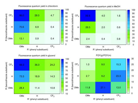
Fig. 3 Heatmaps of the fluorescence quantum yields (%) measured in CHCl<sub>3</sub> (top left), methanol (top right), glycerol (bottom left). The bottom right figure provides the ratio between the glycerol and methanol  $\phi_f$ .
