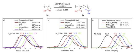
Fig. 2 BV oxidation of PMVKs using high-yielding conditions optimized for the small-molecule model. SEC traces before and after BV oxidations: (a) acid catalyst, mCPBA as oxidant, (b) in the presence of inorganic base, mCPBA as oxidant, (c) MMPP and other peroxyacids as oxidant (see the detailed conditions in Table S3.†).
