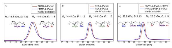
Fig. 6 Synthesis of block copolymers of VAc and various monomers. SEC traces of (a) PMMA-b-PMVK di-block copolymer **7a**, (b) PEA-b-PMVK di-block copolymer **7b** and (c) PMVK-b-PMA-b-PMVK tri-block copolymer **7c** before and after exhaustive BV oxidation.
