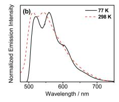
Fig. 4 (a) Emission spectra of 20 wt% 6 doped in the MCP thin film upon increasing the temperature from 160 to 300 K. (b) Normalized PL spectra of the solid sample of 2 at 77 and 298 K.
