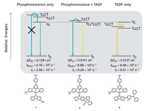
Fig. 5 Relative energies of the excited states involved in the emission (i.e. <sup>3</sup>IL, <sup>3</sup>LLCT and <sup>1</sup>LLCT) of 1, 2 and 6.
