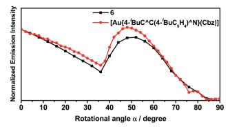
Fig. 6 Angular-dependent PL intensities of the p-polarized light of 6 and  $[Au\{4^{-t}BuC^{\wedge}C(4^{-t}BuC_{6}H_{4})^{\wedge}N\}(Cbz)]$  (11% v/v) in m-CBP thin films with 20 nm thickness.
