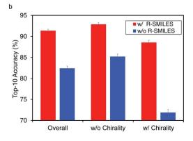
Fig. 4 Accuracies for complex reactions. (a) Top-10 accuracy according to the number of new atoms in reactants. The red and blue lines represent the performance with/without R-SMILES. The gray bar means the percentage of this kind of reaction in the test set. (b) Top-10 accuracy for reactions involving with/without chirality. The red and blue bars represent the performance with or without R-SMILES.
