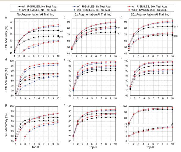
Fig. 2 Top-K accuracy (%) with/without R-SMILES on USPTO-50K for P2R (a)–(c), P2S (d)–(f), and S2R (g)–(i). The solid lines (w/ R-SMILES) and dashed lines (w/o R-SMILES) represent the performance with or without R-SMILES, respectively. The lines with different colors represent the performance in different test set augmentation scenarios.
