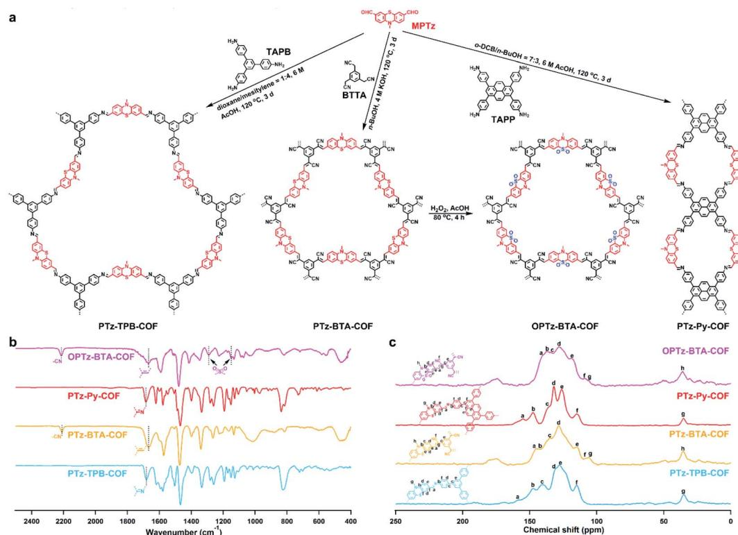
Fig. 1 (a) Synthesis of phenothiazine-based COFs. (b) FT-IR spectra of PTz-TPB-COF, PTz-BTA-COF, PTz-Py-COF, and OPTz-BTA-COF. (c) Solid-state  $^{13}\text{C}$  NMR spectra of PTz-TPB-COF, PTz-BTA-COF, PTz-Py-COF, and OPTz-BTA-COF.
