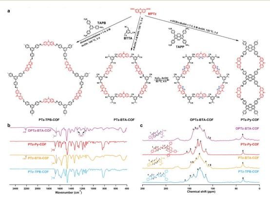
Fig. 1 (a) Synthesis of phenothiazine-based COFs. (b) FT-IR spectra of PTz-TPB-COF, PTz-BTA-COF, PTz-Py-COF, and OPTz-BTA-COF. (c) Solid-state <sup>13</sup>C NMR spectra of PTz-TPB-COF, PTz-BTA-COF, PTz-Py-COF, and OPTz-BTA-COF.
