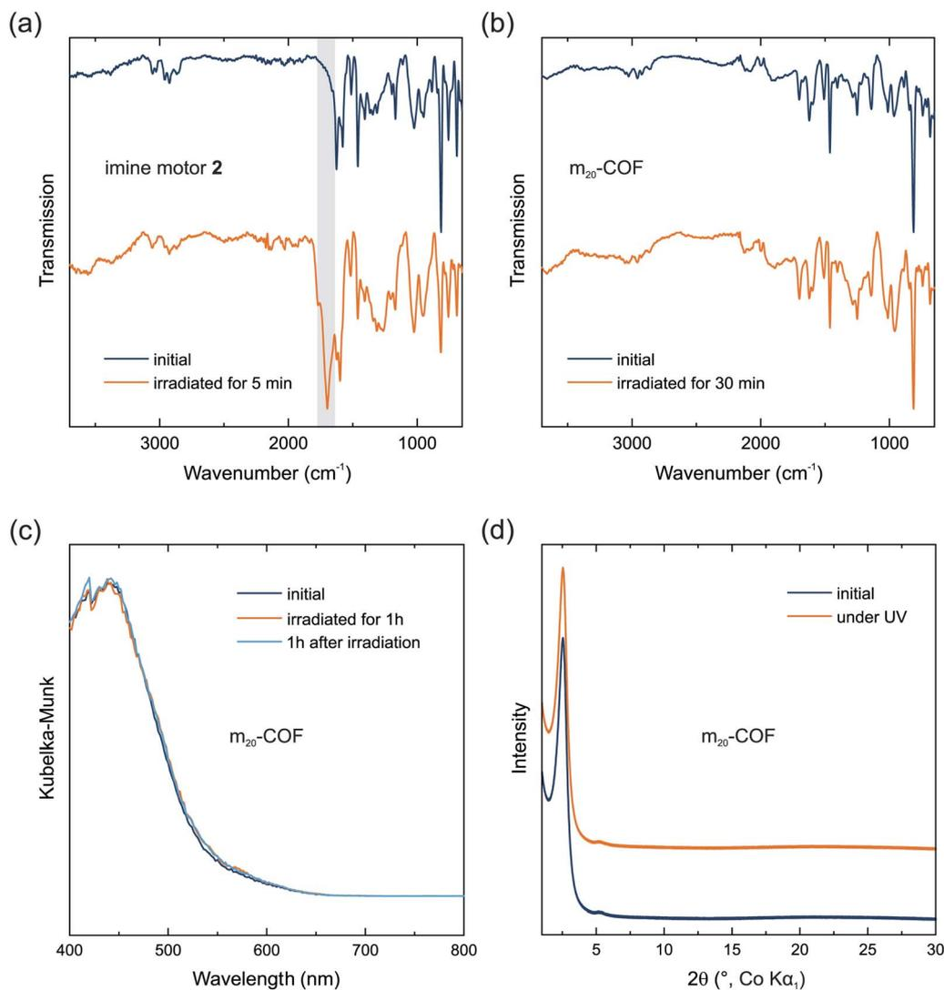
Fig. 5 FT-IR spectra of a thin film of the imine motor 2 (a) and m<sub>20</sub>-COF (b) under prolonged irradiation at 365 nm (UV-LED). Grey area highlights appearing C=O vibrations during irradiation of imine motor 2. Direct reflectance UV/vis spectra (c) and XRPD patterns (d) of m<sub>20</sub>-COF before and during irradiation (>1.5 h) at 365 nm are shown. The patterns are stacked with an arbitrary offset to aid visibility.
