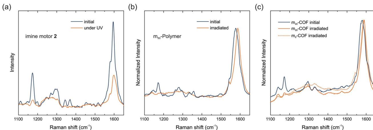
Fig. 4 Raman spectra of the imine motor 2 as a thin-film (a), **m**<sub>50</sub>-P (b), and **m**<sub>20</sub>-COF. The thin-film of the molecular imine motor 2 was recorded at 785 nm and irradiated at 365 nm with a UV-LED. Raman spectra of **m**<sub>50</sub>-P (b), **m**<sub>20</sub>-COF and **m**<sub>0</sub>-COF (c) were recorded with a Raman laser at 355 nm for simultaneous excitation of the motor.
