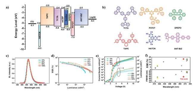
Fig. 4 (a) Device configuration and the energy level diagram. (b) Chemical structures of the materials. (c) EL spectra. (d) EQE *versus* luminance curves. (e) Current density and luminance *versus* voltage characteristics. (f) EQE and FWHM comparison of the reported non-doped blue OLEDs in the literature on the premise of FWHM less than 60 nm.
