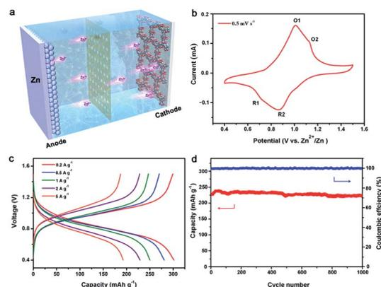
Fig. 3 (a) Illustration of the aqueous Zn/Tp-PTO-COF battery; (b) CV curve at a scan rate of  $0.5 \text{ mV s}^{-1}$ ; (c) galvanostatic charge–discharge curves of the aqueous Zn/Tp-PTO-COF battery at various current densities; (d) cycle stability at a current density of  $2 \text{ A g}^{-1}$ .
