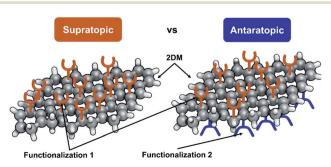
Fig. 1 Schematic representation of Janus 2D materials.
