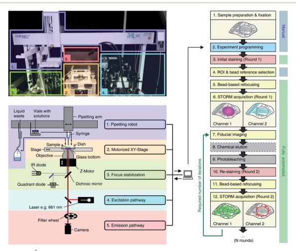
Fig. 5 Automated maS<sup>3</sup>TORM setup and workflow indicating photographic (upper left panel), and schematic outlines (lower left panel) and experimental details for an automated multiplex system (right panel). Reused with permission from ref. 115.
