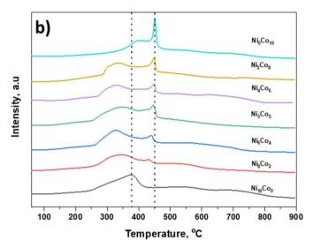
Fig. 1 (a) P-XRD pattern; (b) H<sub>2</sub>-TPR profile of activated carbon supported NiCo-AC catalysts.
