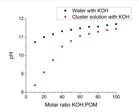
Fig. 3 The pH response of introducing KOH into pure water and 1.0 mg mL $^{-1}$  {Sm $_4$ Nb $_{28}$ } cluster solution.
