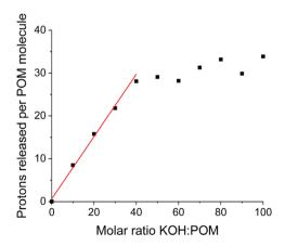
Fig. 4 The number of protons released per molecular cluster (including the protons contributed by the hydrolysis of ammonium ions) versus the molar ratio of KOH introduced to {Sm<sub>4</sub>Nb<sub>28</sub>} clusters.
