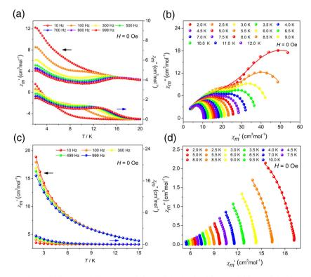
Temperature-dependent  $\chi'$  and  $\chi''$  AC susceptibilities under 0 Oe dc fields for R-1 (a) and R-2 (c); and Cole-Cole plots for R-1 (b) and R-2 (d).
