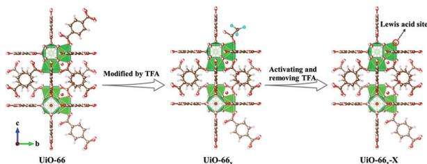
Fig. 1 Schematic illustration of the synthesis of UiO-66<sub>x</sub>-X.
