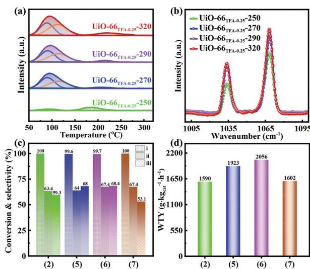
**Fig. 5** (a) NH<sub>3</sub>-TPD of UiO-66<sub>TFA-0.25-X</sub>. (b) FTIR-spectra of pyridine chemisorption on UiO-66<sub>TFA-0.25-X</sub>; the catalytic performance of MN carbonylation to DMC on (2) Pd-UiO-66<sub>TFA-0.25-250</sub>, (5) Pd-UiO-66<sub>TFA-0.25-270</sub>, (6) Pd-UiO-66<sub>TFA-0.25-290</sub> and (7) Pd-UiO-66<sub>TFA-0.25-320</sub>. (c)  $S_{\text{DMC}/\text{CO}}$  (i),  $S_{\text{DMC}/\text{MN}}$  (ii), and  $C_{\text{CO}}$  (iii), and (d) WTY of DMC.
