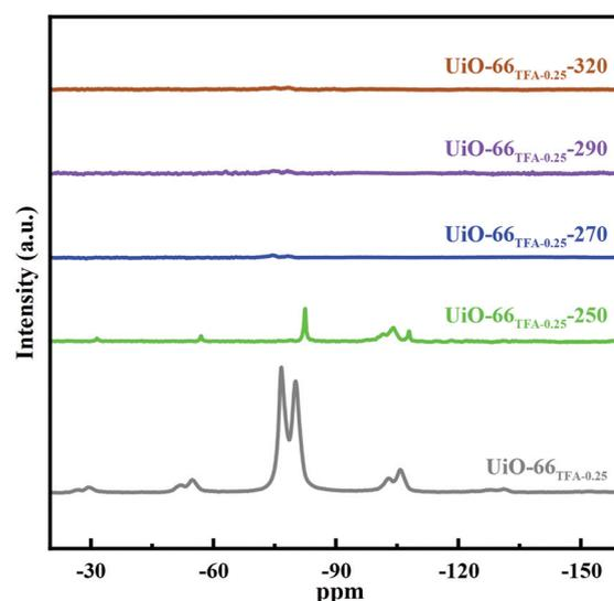
**Fig. 4** Mass-normalized <sup>19</sup>F NMR spectra of UiO-66<sub>TFA-0.25</sub>-X (UiO-66<sub>TFA-0.25</sub>, UiO-66<sub>TFA-0.25</sub>-250, UiO-66<sub>TFA-0.25</sub>-270, UiO-66<sub>TFA-0.25</sub>-290 and UiO-66<sub>TFA-0.25</sub>-320).
