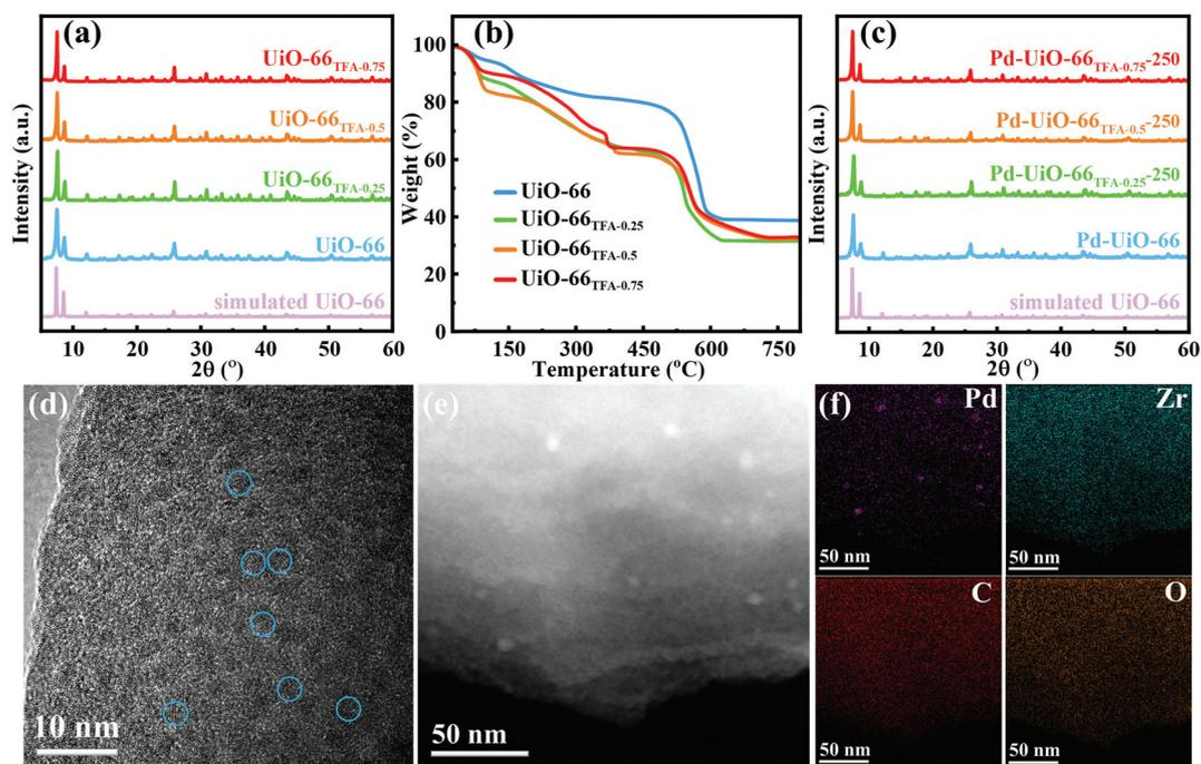
**Fig. 2** (a) XRD patterns of UiO-66<sub>x</sub> (UiO-66, UiO-66<sub>TFA-0.25</sub>, UiO-66<sub>TFA-0.5</sub> and UiO-66<sub>TFA-0.75</sub>); (b) TGA curves of UiO-66<sub>x</sub>; (c) XRD patterns of Pd-UiO-66<sub>x</sub>-250; (d) HTEM image; (e) HAADF-STEM image; and (f) the corresponding Pd, Zr, C, and O elemental mapping of Pd-UiO-66<sub>TFA-0.25</sub>-250.
