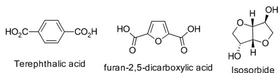
Fig. 10 Comonomers for the synthesis of aromatic-aliphatic copolyesters.
