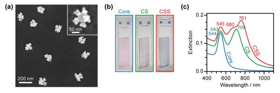
Fig. 2 Structural and optical characteristics of CSS nanoassemblies. (a) Representative SEM image (inset: a magnified view) of CSS nanoassemblies with C8DT as linkers. (b) Photographic images and (c) UV-vis spectra of the Core, CS, and CSS with C8DT as linkers.
