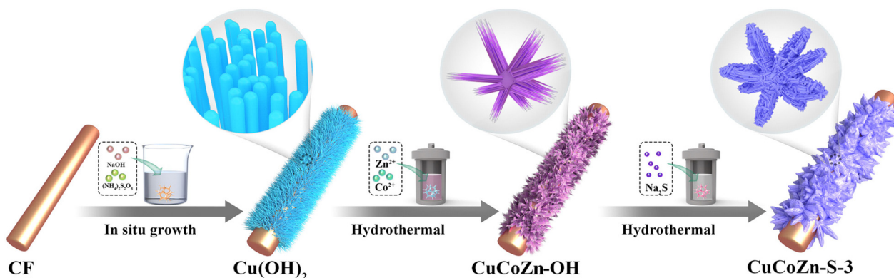
Fig. 1 Schematic diagram of the \text{CuCoZn-S} nanoflower catalyst supported on CF.
