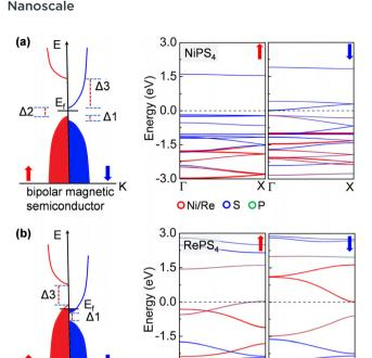
Fig. 3 Electronic band structures of (a)  $NiPS_4$  and (b)  $RePS_4$  nanowires. The contributions from different atoms or orbitals are shown by the colors. The Fermi level is shifted to zero (red dashed lines). The left panels are schematic plots of their band structures.
