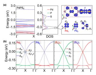
Fig. 4 (a) Electronic band structures and density of states (DOS) of a PdPS $_4$  nanowire calculated without SOC. The right panel displays the partial charge density of the flat band at about -0.3 eV. (b) Band structure of a PdPS $_4$  nanowire calculated with SOC. The contributions from different atoms or orbitals are shown by the colors. The Fermi level is shifted to zero (dashed lines).
