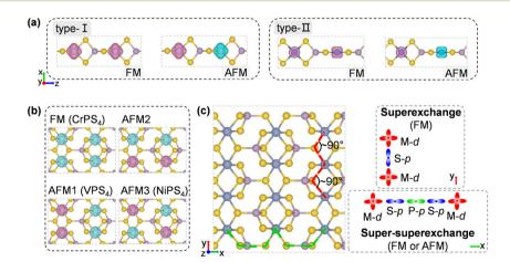
Fig. 6 (a) and (b) Spin density distributions of an MPS<sub>4</sub> nanowire and MPS<sub>4</sub> monolayer in FM and low-energy AFM states. The ground-state magnetic configuration is indicated for VPS<sub>4</sub>, CrPS<sub>4</sub>, and NiPS<sub>4</sub> monolayers, respectively. (c) Schematic illustration of superexchange and super-superexchange interactions for the MPS<sub>4</sub> monolayer.
