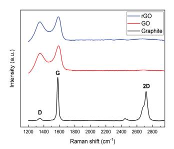
Fig. 2 Raman spectra of graphite, GO and rGO.
