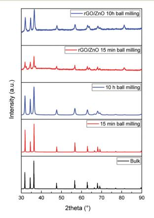
Fig. 3 XRD patterns of bulk and ball milled ZnO nanoparticles as well as the rGO and ZnO hybrid composite materials.
