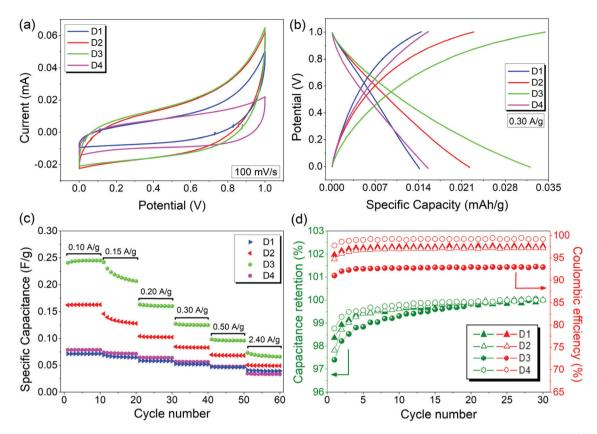
Fig. 9 Electrochemical performances of supercapacitors D1, D2, D3 and D4 with a 6 M KOH electrolyte: (a) CV taken at a 100 mV s<sup>-1</sup> scan rate, (b) charge–discharge curves cycled between 0 and 1 V at a current density of 0.30 A g<sup>-1</sup>, (c) specific capacitances at various current densities, and (d) comparison of the capacitance retention of D1, D2, D3 and D4.
