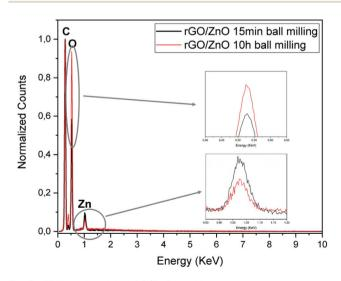
Fig. 5 EDX results of the rGO/ZnO hybrid composite.
