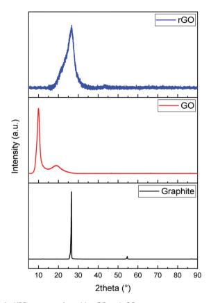
Fig. 1 XRD patterns of graphite, GO and rGO.
