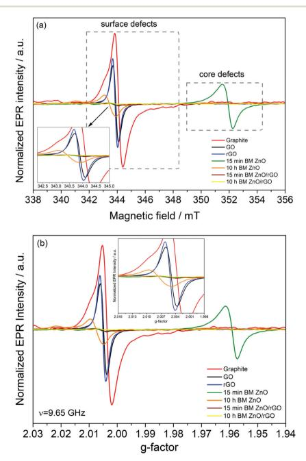
Fig. 7 Room temperature X-band EPR spectra (a) and corresponding g-values (b) of the starting materials and the synthesized powders for supercapacitor electrodes. The EPR intensities are normalized according to the mass of each sample. All EPR measurements were performed under the same conditions with the same parameters (i.e., the same receiver gain, scan number, modulation frequency, modulation amplitude, time constant and microwave power).
