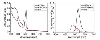
Fig. 4 Optoelectronic properties of layered hybrid perovskites. (a) UVvis absorption spectra and (b) PL spectra of thin films based on (PDMA) PbI<sub>4</sub> (black), (F-PDMA)PbI<sub>4</sub>(blue), and (PF)PbI<sub>4</sub> (red) on microscope glass. Further characteristics are shown in the ESI.†
