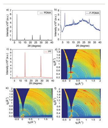
Fig. 2 Structural properties of layered hybrid perovskites. (a-c) XRD patterns of thin films based on (a) (PDMA)Pbl<sub>4</sub> (black), (b) (F-PDMA)Pbl<sub>4</sub> (blue), and (c) (PF)PbI<sub>4</sub> (red) compositions on microscope glass. (d-f) GIWAXS patterns of thin films of (d) (PDMA)PbI<sub>4</sub>, (e) (F-PDMA)PbI<sub>4</sub>, and (f) (PF)PbI<sub>4</sub>. Methods and further analysis is provided in the ESI.†
