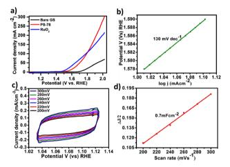
Fig. 3 (a) Polarization curves of PS-78 and the substrate (GS) at a scan rate of 5 mV s<sup>-1</sup>, (b) Tafel plot of PS-78, (c) cyclic–voltammetry curves of PS-78 at different scan rates (200–300 mV s<sup>-1</sup>) and (d) double layer charge capacitance ( $C_{\rm cl}$ ) of PS-78.
