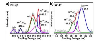
Fig. 5 XPS of PS-78 post OER. The high resolution spectra of (a) Ni 2p and (b) W 4f. The dotted curve demonstrates the experimental data, while the solid line displays the results of fitting.
