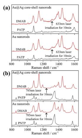
Fig. 2 SERS spectral changes after monochromatic light irradiation for 10 min of (a) PATP adsorbed on the surface of Au nanorods and Au@Ag core-shell nanorods and (b) PNTP adsorbed on the surface of Au nanorods and Au@Ag core-shell nanorods.
