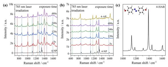
Fig. 7 (a) SERS spectral evolution irradiated with 785 nm monochromatic light: (a) 4-NP adsorbed on Au@Ag core—shell nanorods; (b) 4-NP adsorbed on Au@Ag core—shell nanorods after adding NaBH<sub>4</sub>. (c) Simulated Raman spectrum of 4-HAB molecules and the optimized molecule structures (B3LYP/6-31+G(d)).
