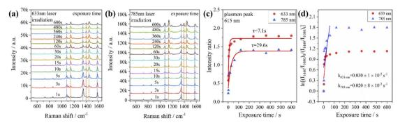
Fig. 4 SERS spectral evolution of PNTP adsorbed on Au@Ag core—shell nanorods irradiated with (a) 633 nm and (b) 785 nm laser wavelengths. (c) The time-dependent relative intensity ratios between the 1440 cm<sup>-1</sup> shift of DMAB and the 1080 cm<sup>-1</sup> shift of PNTP. (d) Plots of  $\ln[(l_{1440}/l_{1080})_0/(l_{1440}/l_{1080})_0]$  versus time for the reduction of PNTP with Au@Ag core—shell nanorods.
