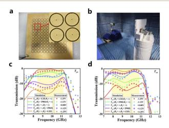
Fig. 5 (a) Photograph of the reconfigurable chiral metasurface. (b) Photograph of the experiment environment. Comparison of measured and experimental transmission spectra for cross-polarization (c)  $T_{vx}$ and co-polarization (d)  $T_{xx}$  for the fabricated metasurface sample in different states.
