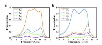
Fig. 2 Transmission coefficient of the linearly polarized wave under normal incidence along the z-axis with different sets of the two paired PIN diode: state 1 (a) and state 2 (b).
