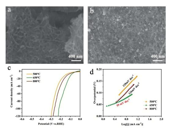
Fig. 5 SEM images of  $MoS_2/MXene/NF$  after sulfurization at (a) 500 °C and (b) 800 °C. (c) Polarization curves and (d) corresponding Tafel plots of  $MoS_2/MXene/NF$  sulfurized at different temperatures.
