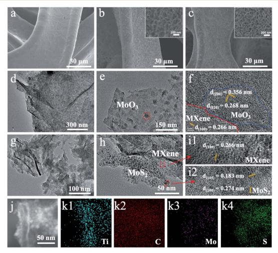
Fig. 2 SEM images of (a) NF, (b)  $MOO_3/MXene/NF$ , and (c)  $MOS_2/MXene/NF$ . The insets of (b and c) are images at high magnification. (d and e) TEM images, and (f) HRTEM image of  $MOO_3/MXene/NF$ . (g and h) TEM images, (i) HRTEM image, (j) HAADF image, and (k) EDX elemental distributions of  $MOS_2/MXene/NF$ .
