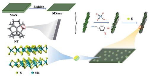
Fig. 1 Schematic diagram of the MoS<sub>2</sub> NDs/MXene/NF synthetic route.
