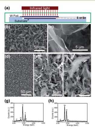
Fig. 1 (a) Schematic diagram of the infrared-heating CVD setup. (b) and (c) SEM images of the film grown with S. (d)—(f) SEM images of film grown with Se. (g) EDS spectrum of the film grown with S. (h) EDS spectrum of the film grown with Se.
