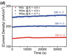
Fig. 6 (a) LSV curves measured on working electrodes of  $WSe_2$  nanosheets,  $WS_2$  nanosheets, or Pt for the HER in acid. The inset shows a digital photo of a  $WSe_2$  thin film working electrode. (b) EIS Nyquist plots and (c) Tafel plots of different catalyst working electrodes. (d) Stability plots recorded on  $WSe_2$  thin film or  $WS_2$  thin film catalysts at different high-current levels.
