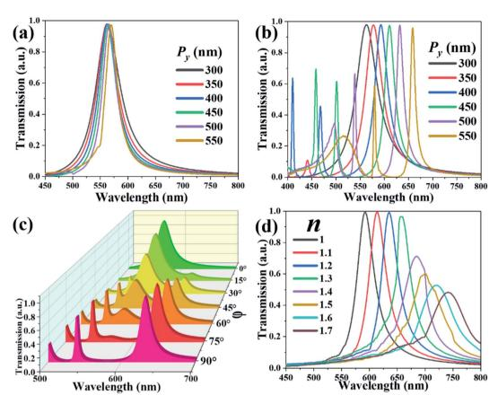
Fig. 6 Transmission spectra of TCF-2 with different  $P_y$  values from 300 nm to 550 nm at normal incidence in (a) TE and (b) TM modes. Transmission spectra of TCF-2 (c) with different  $\varphi$  values at the normal incidence and (d) exposed to the ambient environment with different n values under the condition of  $P_x = 300$  nm and  $P_y = 500$  nm under normal TE-polarized incident light.
