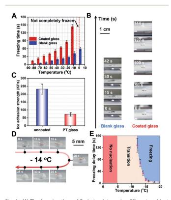
Fig. 4 (A) The freezing time of 5  $\mu$ L droplets under different ambient temperature conditions. (B) The process of 5 µL droplets freezing on the surface of coated glass and blank glass at -10 °C. (C) Ice adhesion strength of blank glass and photothermal coating. (D) The process of 5 μL droplet freezing under light conditions at an ambient temperature of -14 °C. (E) Time taken for droplets to freeze completely under different room temperature conditions at one solar illumination.
