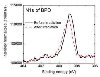
Fig. 3 N1s spectra of the BPD SAM before (solid-black curve) and after (dashed-red curve) electron irradiation.
