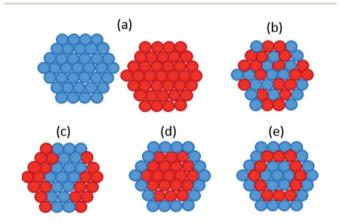
Different possible atomic structures of bimetallic nanoparticles (a) separate monometallic nanoparticles; (b) mixed alloys; (c) clusterin-cluster; (d) core-shell; (e) multishell.
