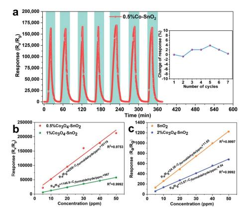
Fig. 9 (a) The seven-time continuous cycle curve of the 0.5%Co-SnO<sub>2</sub> NPs to 30 ppm formaldehyde at 90 °C and the change of response after continuous repetition, (b) the linear fitted curves between concentration and response of 0.5%Co-SnO2 NPs and 1%Co-SnO2 NPs, (c) the linear fitted curves between concentration and response of SnO<sub>2</sub> NPs and 2%Co-SnO<sub>2</sub> NPs
