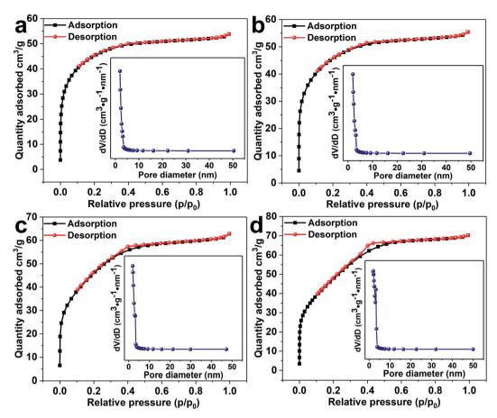
Fig. 5 Nitrogen adsorption—desorption isotherms and corresponding pore size distribution (inset) of (a) SnO<sub>2</sub> NPs, (b) 0.5%Co-SnO<sub>2</sub> NPs, (c) 1% Co-SnO<sub>2</sub> NPs and (d) 2%Co-SnO<sub>2</sub> NPs.
