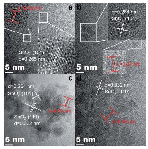
Fig. 4 (a-d) The HRTEM images of SnO<sub>2</sub> NPs, 0.5%Co-SnO<sub>2</sub> NPs, 1%Co-SnO<sub>2</sub> NPs and 2%Co-SnO<sub>2</sub> NPs.
