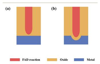
Fig. 6 (a) Schematic of FAD theoretical expectations and (b) schematic of the experimental phenomena.
