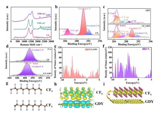
Fig. 2 Raman spectra (a) from pristine CF<sub>x</sub>, GDY and CF<sub>x</sub>/GDY. C 1s and F 1s spectra of CF<sub>x</sub> (b and d), GDY (c) and CF<sub>x</sub>/GDY (c and d). Total densities of states of CF<sub>x</sub> (e) and CF<sub>x</sub>/GDY (f) and the corresponding electron density differences (g and h), respectively, and the corresponding schematic diagram (i).
