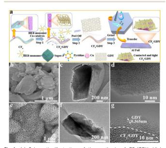
**Fig. 1** (a) Schematic illustration of the synthesis of  $CF_x/GDY$ . High-resolution SEM images of  $CF_x$  (b) and  $CF_x/GDY$  (e). TEM images (c and f) and HRTEM images (d and g) of  $CF_x$  and  $CF_x/GDY$ , respectively.
