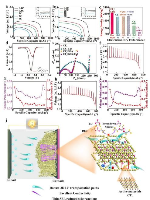
Fig. 3 (a and b) Rate performances of  $CF_x$  and  $CF_x/GDY$  hybrids. (c) Comparison of energy densities of  $CF_x/GDY$  with the reported literature. (d) Cyclic voltammetry profiles and (e) the electrochemistry impedance spectra (EIS). The GITT curves of  $CF_x$  (f) and  $CF_x$ /GDY hybrids (h) and the related voltage and ohmic polarization curves derived from the GITT plots of various electrodes (g and i). (j) Schematic illustration of the reaction mechanism for CF<sub>x</sub>/GDY hybrids
