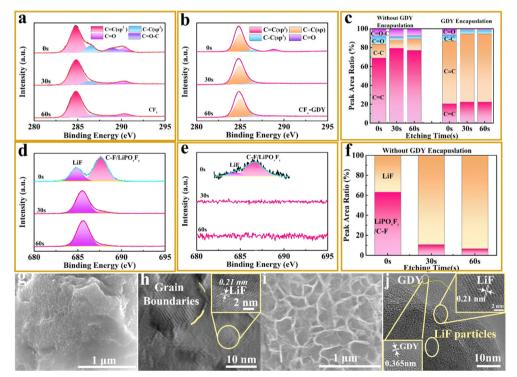
Fig. 4 C XPS spectra (a and b), F spectra (d and e) and the relative contents (c and f) stemming from the different depths given in Fig. (a and b) and (d and e) of CF<sub>x</sub> and CF<sub>x</sub>/GDY hybrids at the discharge state of 1.5 V, respectively. The SEM images (g and i) and HRTEM images (h and j) of CF<sub>x</sub> and CF<sub>x</sub>/GDY hybrids, respectively
