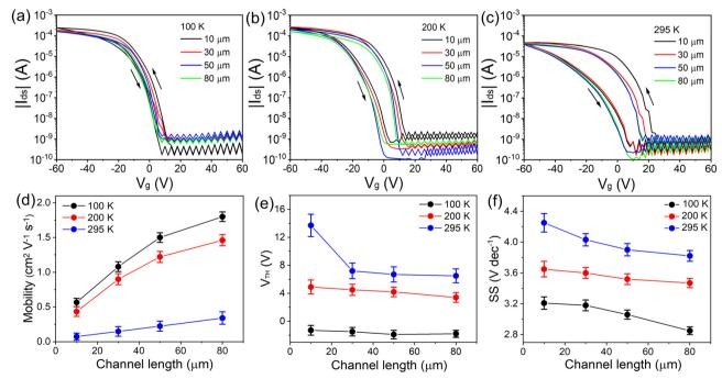
Fig. 6 Transfer characteristics measured at (a) 100 K, (b) 200 K, and (c) 295 K of 120 °C hot-casting (TEA)<sub>2</sub>SnI<sub>4</sub> FETs with different channel lengths L from  $10-80 \mu m$  and constant  $W = 1000 \mu m$ . (d) Average charge carrier mobility, (e) threshold voltage, and (f) subthreshold swing as a function of channel length measured for (TEA)<sub>2</sub>SnI<sub>4</sub> FETs at 100 K, 200 K and 295 K. The error bars were calculated from 12 devices.
