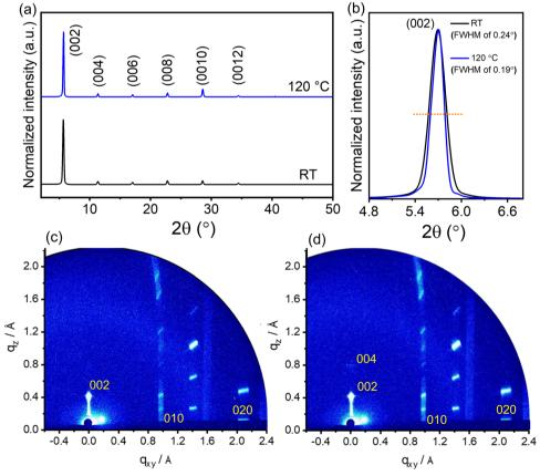
Fig. 3 (a) Out-of-plane XRD measured for  $(TEA)_2SnI_4$  thin films cast at RT and 120 °C. (b) FWHM analysis of the (002) peak. GIWAXS patterns for  $(TEA)_2SnI_4$  cast at (c) RT and (d) 120 °C (reflections are assigned by Miller indices).
