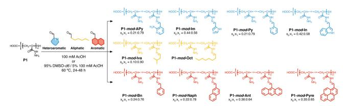
Scheme 2 Synthesis of functional polymers P1-mod-aldehyde, and list of polymers prepared with aldehyde conversions
