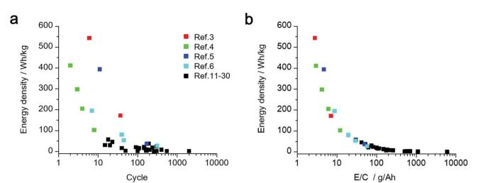
Fig. 2 Estimated cell-level energy density of the LAB reported in the literature. (a) Relationships between energy density and cycle life of LAB. (b) Relationships between energy density and the ratio of the electrolyte weight to cell capacity  $(E/C, g A^{-1} h^{-1})$ .
