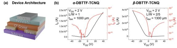
Fig. 2 (a) The bottom-contact, top-gate transistor architecture used to extract the trap-DOS for each polymorph. (b) Examples of transfer characteristics in the linear regime for each polymorph. The  $V_{DS}$ , channel dimensions as a ratio of length to width (L/W), and thickness of the parylene-N gate dielectric (tPary) are given in the inset.
