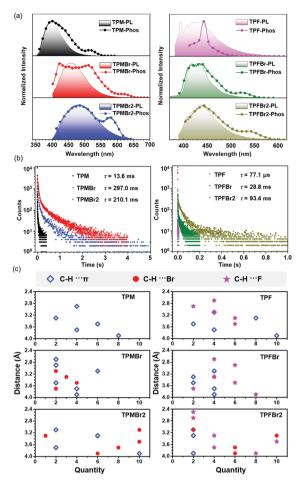
Fig. 4 (a) Photoluminescence and RTP spectra of triphenylethylene derivatives. (b) RTP decay of triphenylethylene derivatives. (c) The distance and quantity of intermolecular interactions of triphenylethylene derivatives from each molecule with adjacent ones in single crystals.
