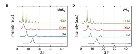
Fig. 3 XRD of the n-alkylamine intercalated (a) MoS<sub>2</sub> and (b) WS<sub>2</sub>. Green: hexadecylamine-intercalated; red: dodecylamine-intercalated; blue: octylamine-intercalated; dark gray: restacked.
