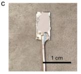
Fig. 1 (a) Optical image of a representative restacked MoS<sub>2</sub> film on a nitrocellulose membrane. (b) SEM cross sectional image of a representative restacked MoS<sub>2</sub> film. (c) Optical image of an electrode prepared by transferring a restacked MoS<sub>2</sub> film onto a gold substrate. The edges of the electrode were sealed using silver paint.
