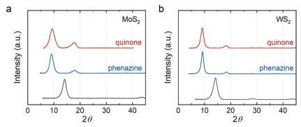
Fig. 4 XRD of electron-proton transfer mediator intercalated (a) MoS<sub>2</sub> and (b) WS<sub>2</sub>. Red: p-benzoquinone-intercalated; blue: phenazine-intercalated; dark gray: restacked.
