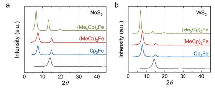
Fig. 2 XRD of metallocene intercalated (a) MoS<sub>2</sub> and (b) WS<sub>2</sub>. Green: decamethylferrocene-intercalated; red: 1,1'-dimethylferrocene-intercalated; blue: ferrocene-intercalated; dark gray: restacked.
