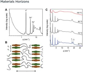
Fig. 3 (A) 1D transmission scattering profile of Pyr-Si<sub>8</sub>-NDI at room temperature. (B) Schematic representation of the room temperature packing of Pyr-Si<sub>8</sub>-NDI. (C) Variable temperature 1D transmission scattering profile of Pyr-Si<sub>8</sub>-NDI upon heating.
