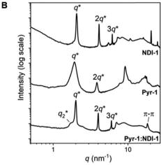
Fig. 1 (A) DSC trace (second heating and cooling cycle) of **Pyr-1:NDI-1**. A temperature ramp of 10 K min<sup>-1</sup> was used. Endothermic heat flows have a positive value. (B) 1D transmission scattering profiles of **Pyr-1:NDI-1** (bottom), **Pyr-1** (middle) and **NDI-1** (top) at room temperature.
