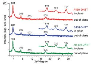
Fig. 3 Out-of-plane and in-plane XRD patterns of spin-coated (a) and vacuum-deposited (b) thin films on OTS-treated substrates.
