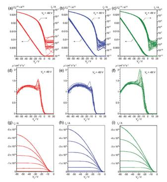
Fig. 4 Transfer curves (a-c), gate-voltage-dependence of mobility (d-f), and output curves (g-i) of OFET devices based on vacuum-deposited R- (red), S- (blue), and rac- (green) EH-DNTT thin films, respectively. Transfer and gate-voltage-dependent mobility curves are overlaid for more than twelve devices.
