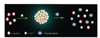
Scheme 1 Schematic representation of the possible mechanism of quenching of the delayed bright green luminescence of Zn Au NCs upon the addition of sodium pyrophosphate.
