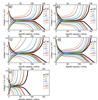
Fig. 7 Initial galvanostatic discharge/charge profiles at different C-rates for the mesoporous LTO-A-600 (a), LTO-A-700 (b), LTO-B-600 (c), LTO-B-700 (d) and LTO-C-700 (e)
