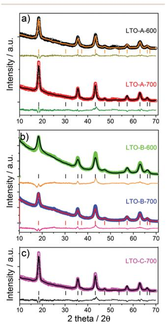
Fig. 2 XRD patterns of the mesoporous LTO microspheres listed in Tables 1 and 2, (a) LTO-A, (b) LTO-B and (c) LTO-C. The symbols show the experimental data and the lines are fitted Rietveld refinements. The vertical bars indicate the tabulated peak positions for spinel LTO, below which the differences between experimental data and fits are plotted. In (c) the peaks expected for a spinel structure (space group: Fd3m) are indexed with the (hkl) values of the corresponding lattice planes
