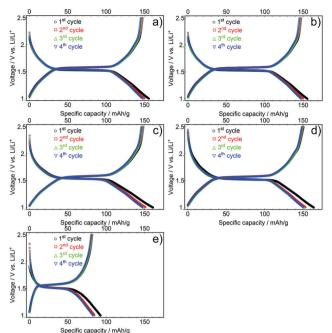
Fig. 6 First four galvanostatic discharge and charge profiles of mesoporous LTO-A-600 (a), LTO-A-700 (b), LTO-B-600 (c), LTO-B-700 (d) and LTO-C-700 (e), C-rate of 0.5.
