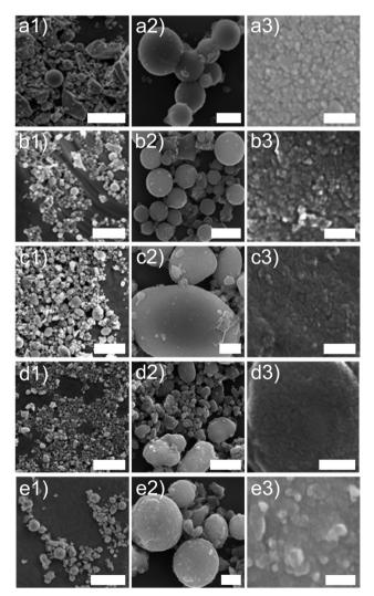
Fig. 4 Low to high magnification SEM images (left to right columns) of mesoporous LTO-A-600 (a), LTO-A-700 (b), LTO-B-600 (c), LTO-B-700 (d), and LTO-C-700 (e) showing the predominance of LTO spheres exhibiting mesoporosity. Left column scale bar: 20 μm, centre column scale bar: 2 µm, right column scale bar: 100 nm.
