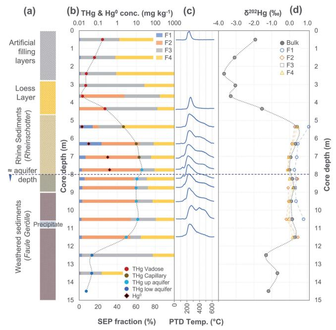
Fig. 6 Multi-analyses summation of SCB3 solid-phase material. (a) Description of approximate soil core layer profile is based on our own visual characterisation and literature descriptions.  $^{53-55}$  (b) THg and Hg $^0$  concentration (logarithmic scale) and SEP speciation data. (c) PTD speciation data – all signal attenuations are normalised to the maximum attenuation for each sample. (d)  $\delta^{202}$ Hg (MDF) stable isotope data.
