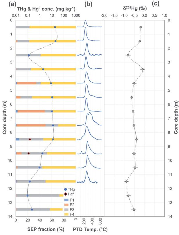
Fig. 2 Multi-analyses summation of SCA1 solid-phase material. (a) THg and Hg<sup>0</sup> concentration (logarithmic scale) and SEP speciation data. (b) PTD speciation data – all signal attenuations are normalised to the maximum attenuation for each sample. (c)  $\delta^{202}$ Hg (MDF) stable isotope data of the bulk sample. Aquifer depth could not be estimated as there were no adjacent wells to this soil core at the same elevation.
