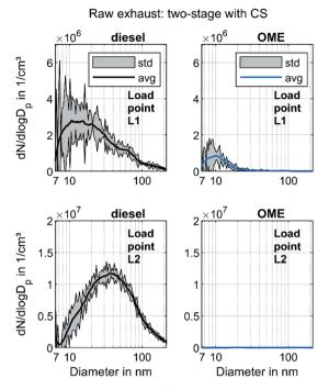
Fig. 4 Particle size distributions of OME and diesel raw exhaust with volatile particle remover and two-stage dilution: filtered average (arithmetic mean) of three recordings and indication of the standard deviation
