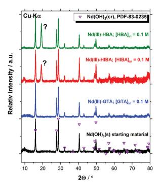
Fig. 9 XRD patterns of the Nd(III) solid phase used as starting material, and the corresponding solid phases after equilibration in the solubility experiments with GTA, HIBA and HBA at  $[L]_{tot} = 0.1$  M. Symbols reproduce the patterns reported for Nd(OH)<sub>3</sub>(cr) (PDF-83-0235) reference material.
