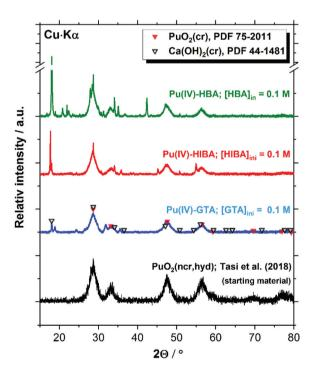
Fig. 10 XRD patterns of the Pu( $_{\rm IV}$ ) solid phase used as starting material (as reported in (Tasi *et al.*, 2018), and the corresponding solid phases after equilibration in the solubility experiments with GTA, HIBA and HBA at [L]<sub>tot</sub> = 0.1 M, in all cases containing HQ as redox buffer. Symbols reproduce the patterns reported for PuO<sub>2</sub>(cr) (PDF-75-2011) and portlandite (Ca(OH)<sub>2</sub>(cr), PDF-44-1481) reference materials.
