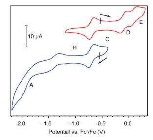
Fig. 2 Cyclic voltammograms of 1 in a 0.15 M solution of TBAPF<sub>6</sub> in THF under N2. Black tick marks indicate open circuit potentials. A, B, C, D, and E mark, respectively, the dominant species within the  $[Ni_3(HITP^{n-})]$  series (n = 5, 4, 3, 2, 1).
