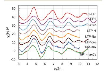
Fig. 8 Fit of titanium K edge EXAFS data of titanium(IV) phosphates, experimental – colored lines, models with structure parameters (in Table 3) – red lines, sample 2 –  $\alpha$ -TiP, sample 1 – TiP1-H, sample 4 – aTiP, sample 3 – LTP-H, sample 5 – LTP-Na sample 6 – LTP-pro, sample 9 – TiP1-mix, and sample 10 – TiP1-mixCa, and (sample 7 – data of insufficient quality, and no data available for sample 8). The offset between the spectra is 8.
