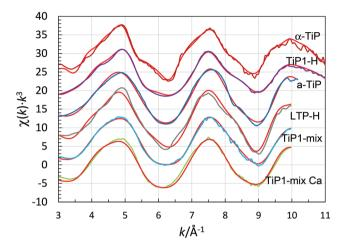
Fig. 5 Fit of phosphorus K edge EXAFS data of titanium(IV) phosphates, experimental - coloured lines, models with structure parameters from Table 4 - red lines, sample 2 -  $\alpha$ -TiP (offset: 30), sample 1 - TiP1-H (offset: 24), sample 4 - aTiP (offset: 18), sample 3 - LTP-H (offset: 12), sample 9 - TiP1-mix (offset: 6), and sample 10 - TiP1-mixCa (no offset).
