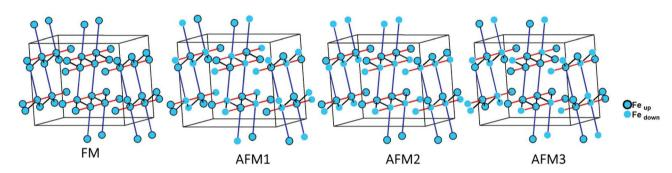
Fig. 4 Different magnetic configurations of  $Ba_5Fe_2In_4Zn_1S_{15}$  used in the DFT+U calculations; J1, J2 and J3 are represented in black, red and blue, respectively.
