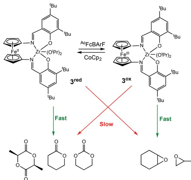
**Scheme 3** A zirconium complex bearing a fully conjugated ligand for the preferential ROP of several cyclic esters and epoxides.<sup>24</sup>
