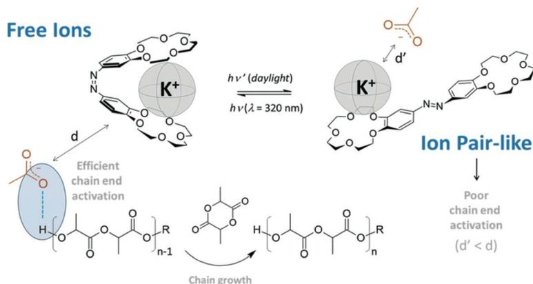
**Fig. 8** A photoresponsive azobenzene incorporated bis(15-crown-5-ether) which transforms the  $K^+OAc$  ion pair like into free ions through a butterfly movement by *E/Z* isomerisation of the azo linkage resulting in increased polymerisation rates.<sup>100</sup> Reproduced from ref. 100 with permission from Royal Society of Chemistry.
