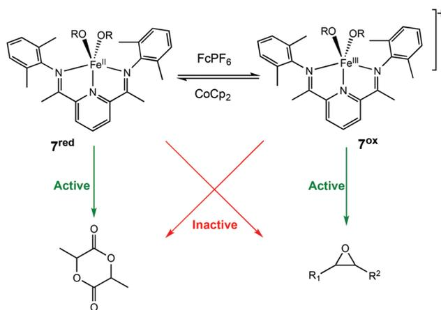
**Scheme 6** Redox switchable Iron(II)/(III) complexes for ROP of LA and CHO.<sup>44</sup>
