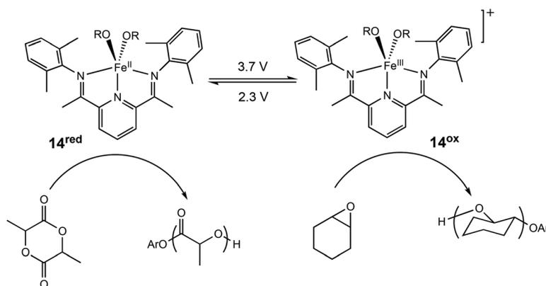
**Scheme 8** Electrochemically switchable ROP of CHO and LA with a bis(imino)pyridine iron alkoxide complex.<sup>11,14</sup>
