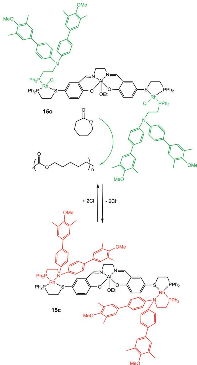
**Scheme 9** Allosteric control of a triple-layer Al(III)-salen catalyst for ROP of CL.<sup>65</sup>
