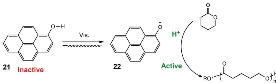
Scheme 14 ROP catalysed by PyOH under light to generate a stronger acid.<sup>87</sup>
