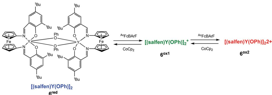
**Scheme 5** A redox switchable dimeric yttrium complex displaying three oxidation states upon stepwise oxidation leading to a mono-oxidised ( $6^{\text{ox}1}$ ) and a doubly oxidised species ( $6^{\text{ox}2}$ ).<sup>36</sup>
