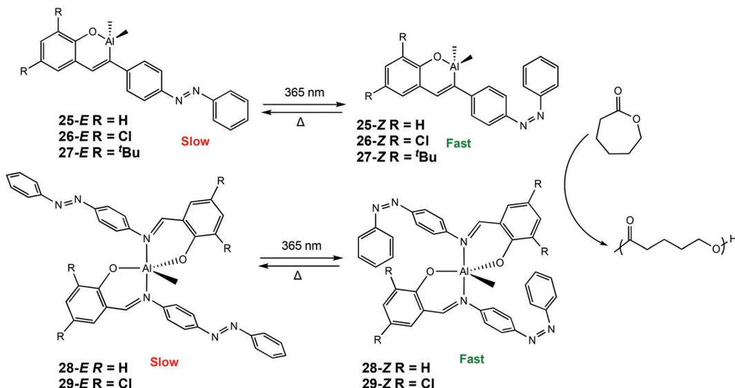
**Scheme 17** Photoswitchable Al(III) complexes bearing azobenzene Schiff-base ligands which undergo *trans*–*cis* isomerisation for ROP of CL.<sup>7</sup>
