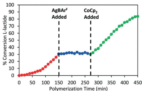
**Fig. 3** Time vs. conversion plot of redox switchable ROP of L-LA using Zr complex **8b**<sup>red/ox</sup>.<sup>50</sup> The oxidised species **8b**<sup>ox</sup> was generated *in situ* by addition of AgBARF (blue circles) and the reduced species was regenerated by CoCp<sub>2</sub> (green circles). Reproduced from ref. 50 with permission from the Royal Society of Chemistry.
